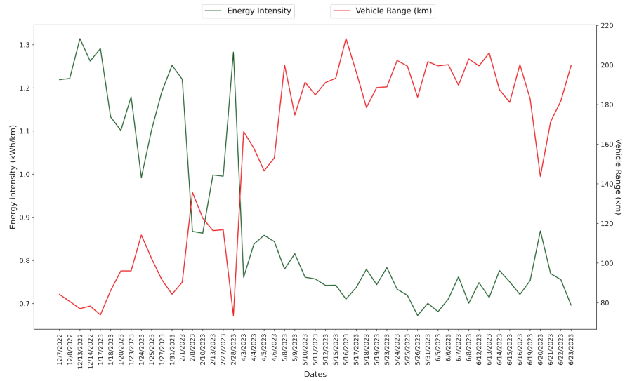
Figure 5: Energy intensity of trips and range implications across days of operations
